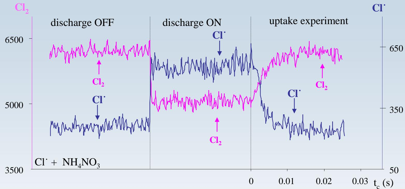
➤ Cl<sub>2</sub> formation by heterogeneous recombination of Cl·
