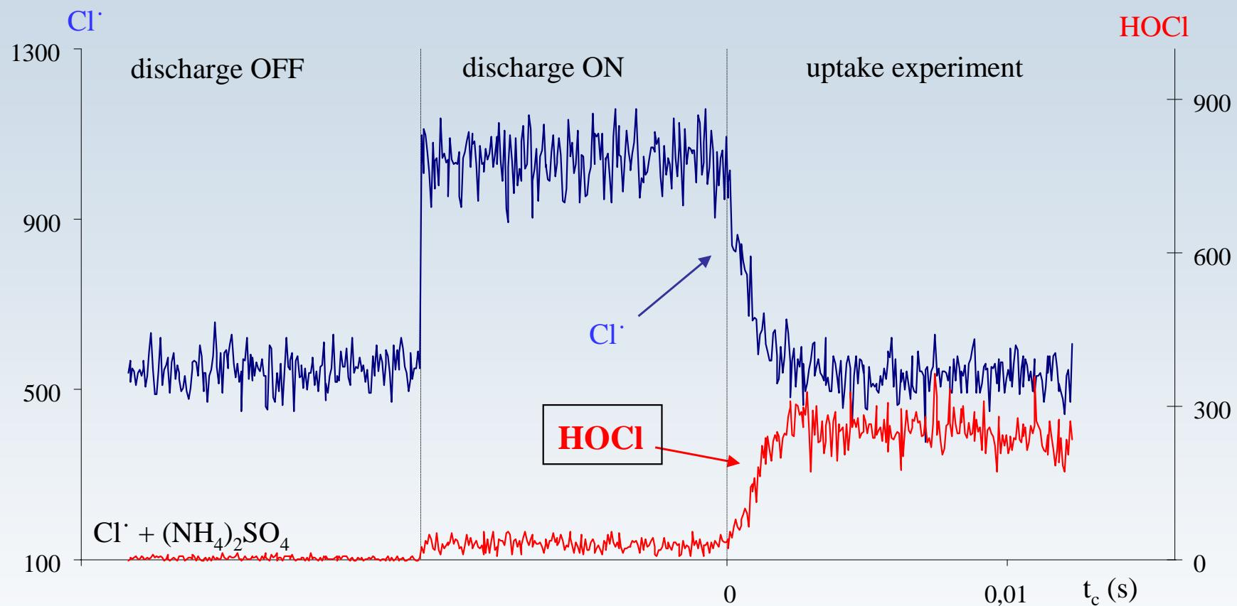
➤ hypochlorous acid formation at low temperatures and in presence of surface adsorbed water
