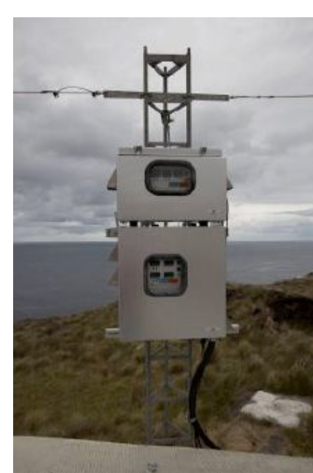
Figure 5. Tekran front-end modules 1130 and 1135 installed on the roof Pointe Bénédicte's laboratory at Amsterdam Island (37.79604°S, 77.55095°E). (from Barret M., A. Dommergue, C.P.
